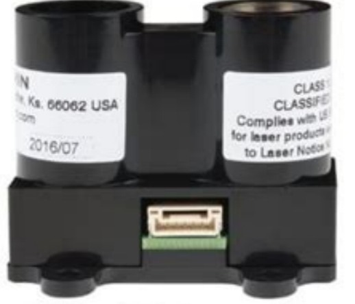
This is the LIDAR-Lite v3, a compact, high-performance optical distance measurement sensor from Garmin
