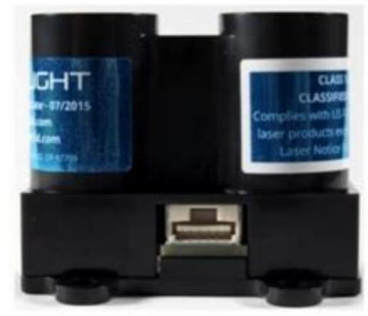
LIDAR-Lite v2, a compact high performance optical distance measurement sensor from PulsedLight.
